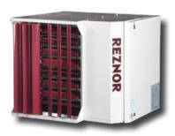
The UDSA (axial fan, free blowing) and UDSBD (centrifugal fan, ducted) achieve 92% thermal efficiency and incorporate a unique 4-pass heat exchanger manufactured from titanium stabilised aluminised steel for enhanced life expectancy.
